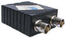
Dual BNC Female RJ45 Part Number: E10120D 2 and 8 Mbps Version
